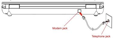
Figure 4-18 Connecting the internal modem
